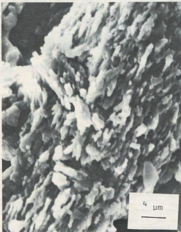
Fig. 5. Scanning electron micrograph of a portion of an individual crystal-like form, showing the morphology of the crystallite bundles.
